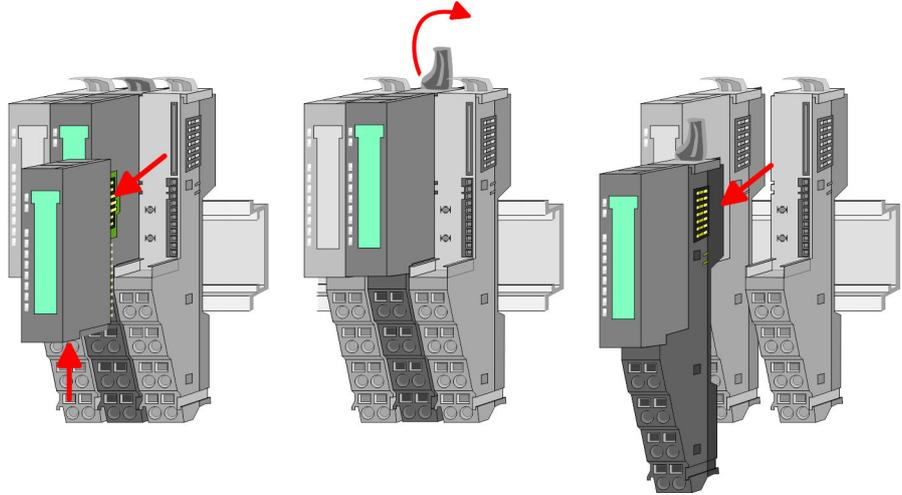
2. ➤ Press the unlocking lever at the lower side of the just mounted right module and pull it forward.
