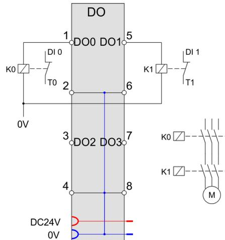
You can connect a load (e.g., a relay) between a digital safety output DO 0 ... 3 and the ground connection 0V of the field power supply. It is not necessary to lead back the ground connection to the according connection of the System SLIO safety module.
