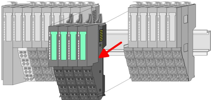
3. ➤ Turn all the locking lever of the module group to be exchanged upwards.
