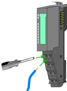
1. ➤ Insert a suited screwdriver at an angle into the square opening as shown. Press and hold the screwdriver in the opposite direction to open the contact spring.
