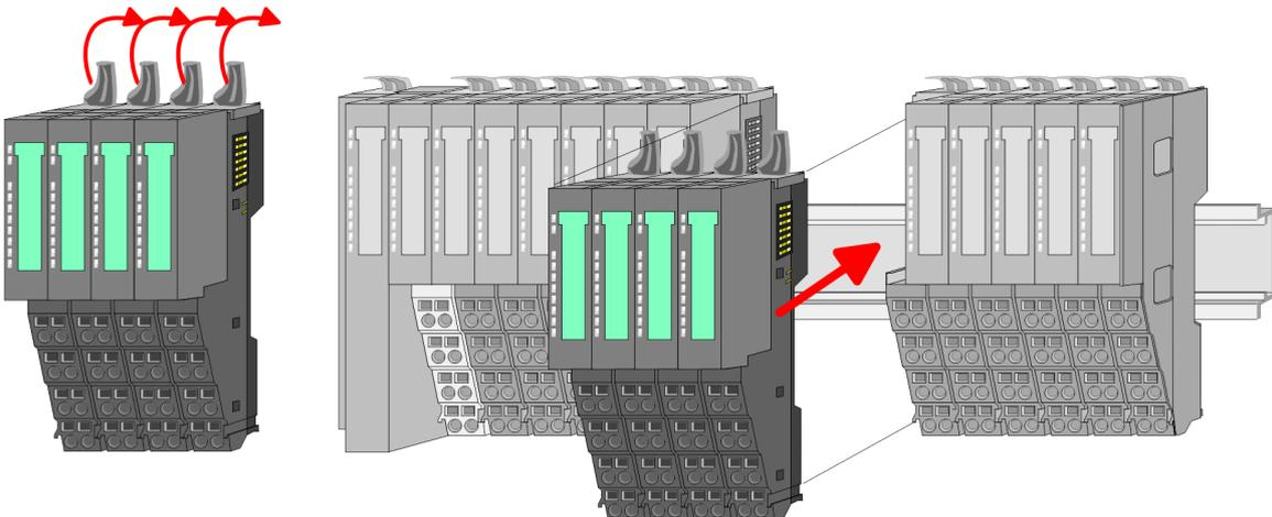
5. ➤ For mounting turn all the locking lever of the module group to be mounted upwards.
