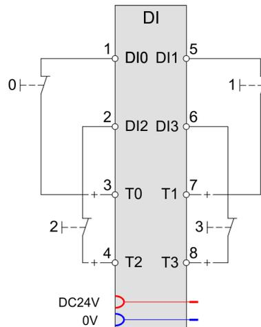
**Connection 4 x emergency off, single-channel, *Test pulse activation* not active**
