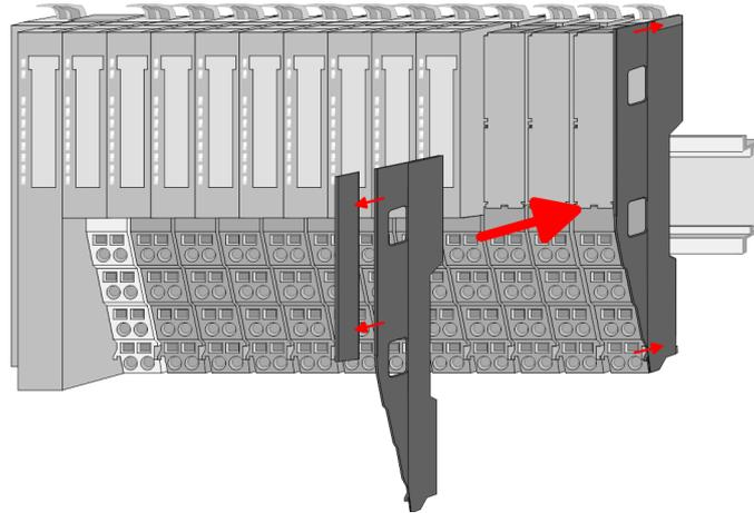
→ If the last module is a clamp module, for adaptation the upper part of the bus cover is to be removed.
