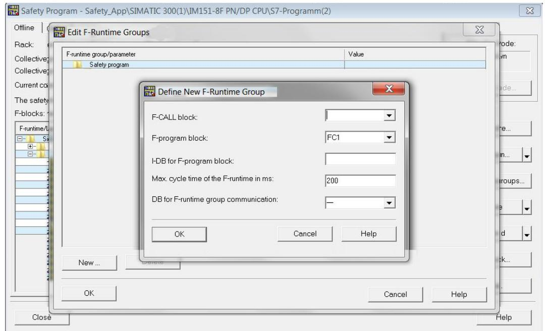
4. ➔ Enter "FC2" at "F\_CALL block". This FC is automatically generated, as soon as you have left the dialog *'Edit F-Runtime groups'* with [OK]. Due to the usage of a FC as F-program block, there is no instance DB (I-DB) required for the F-program block. The max. cycle time of the F-runtime group should be 200ms. A DB for the F-runtime group communication is not required.
