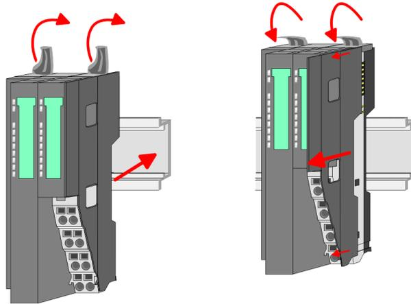
1. → Start at the left side with the head module (e.g. bus coupler). For this turn both locking lever upwards, put the head module to the mounting rail and turn both locking lever downward.
