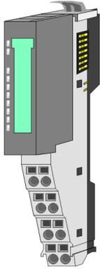
In the System SLIO the power supply is established by *power modules*. These are either integrated to the bus coupler or may be installed between the periphery modules. Depending on the power module isolated areas of the DC 24V power section supply may be defined respectively the electronic power supply may be extended with 2A. For better recognition the color of the power modules are contrasting to the periphery modules.
