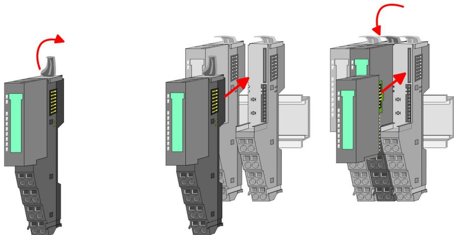
5. ➤ For mounting turn the locking lever of the module to be mounted upwards.
