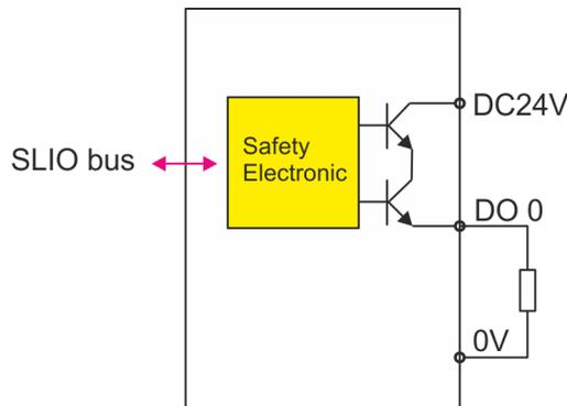
**Connection a load to a safety output**
