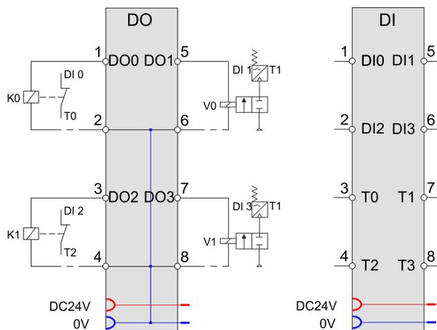
**Connection 2 parallel connected loads to a safety output**
