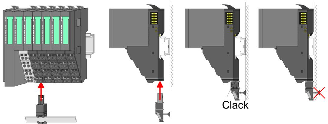
→ The shield bus carrier (available as accessory) serves to carry the shield bus to connect cable shields. The shield bus carrier is mounted underneath the terminal of the terminal module. With a flat mounting rail for adaptation to a flat mounting rail you may remove the spacer of the shield bus carrier.
