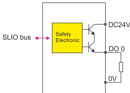
**Connection a load to a safety output**
