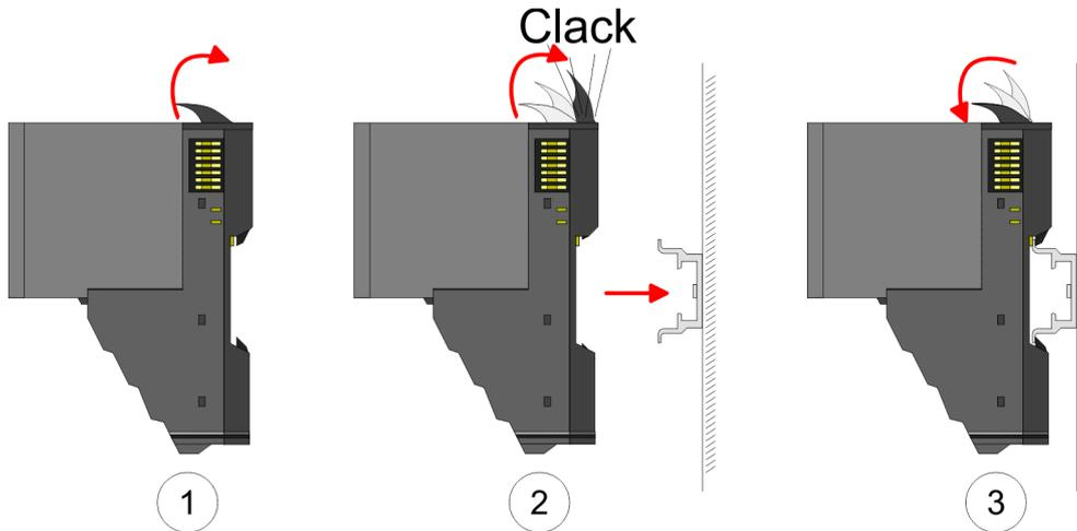
For the exchange of a electronic module, the electronic module may be pulled forward after pressing the unlocking lever at the lower side of the module. For installation plug the electronic module guided by the strips at the lower side until this engages audible to the terminal module.
