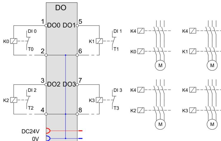
**Connection 2 motors, 2-channel with feedback (2 contactor per motor)**
