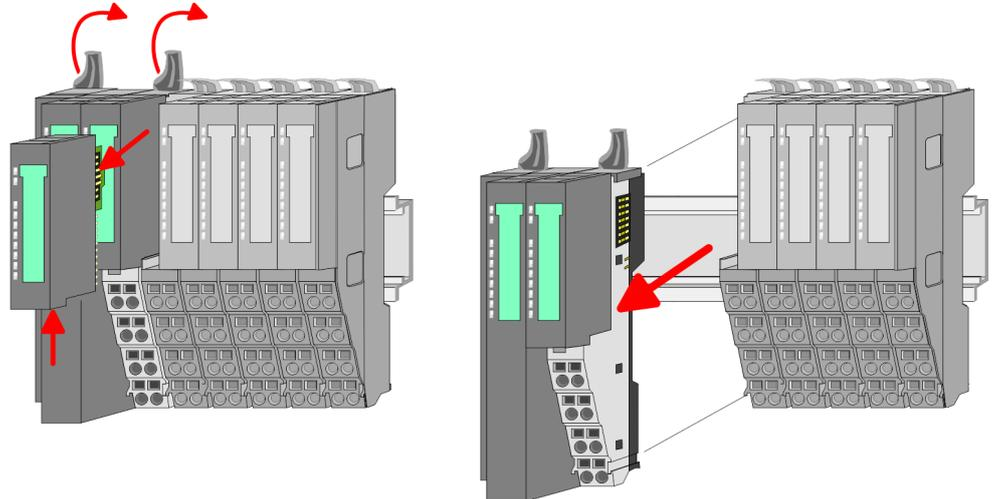
2. Press the unlocking lever at the lower side of the just mounted right module and pull it forward.
