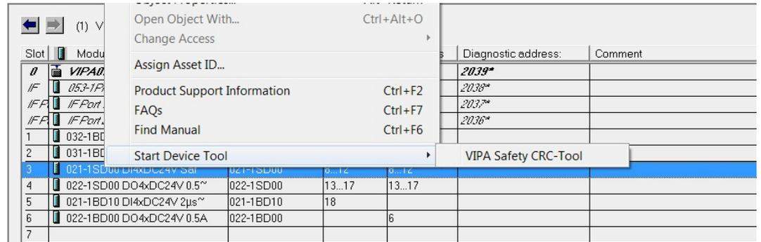
2. Validate each parameter in the CRC-Tool according to the description "Validation of the system" with the [Accepted] button and then calculate the checksum with [Calc-CRC]. The [Calc-CRC] button is only enabled when all the parameters were "accepted". Chapter 3.11 'Validation of the system' on page 114
