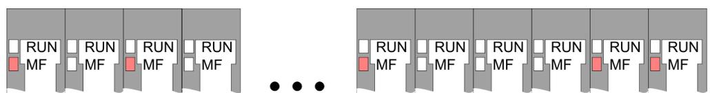
**Behaviour:** After PowerON the RUN LED of each module is off and the MF LED of each module is sporadically on.
