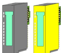
The functionality of a SLIO periphery module is defined by the *electronic* module, which is mounted to the terminal module by a sliding mechanism. With an error the defective module may be exchanged for a functional module with standing installation. At the front side there are LEDs for status indication. For simple wiring each module shows a corresponding connection diagram at the front and at the side.
