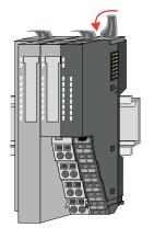
**6.** Turn the locking lever of the periphery module downward, again.
