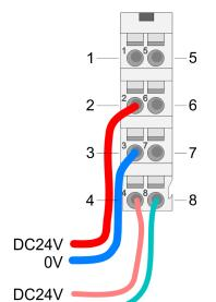
For wires with a core cross-section of 0.08mm<sup>2</sup> up to 1.5mm<sup>2</sup>.
