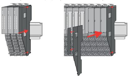
After mounting the whole system, to protect the backplane bus connectors at the last module you have to mount the bus cover, now. If the last module is a clamp module, for adaptation the upper part of the bus cover is to be removed.
