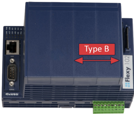
Figure 4. Position of the B Slots on all other Ewon Flexy.
