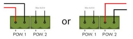
If only one power supply is used, the alarm contact is closed. If two power sources are connected, the contact is open. As soon as one of the power supplies fails, the contact will close and the Power Indicator LED will blink.
