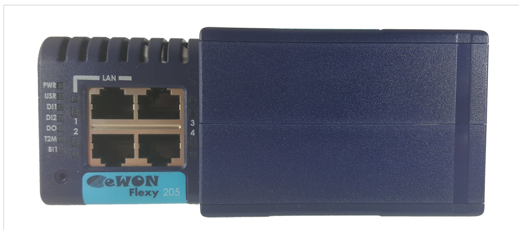
Fig. 10 Interface of the Flexy 205
