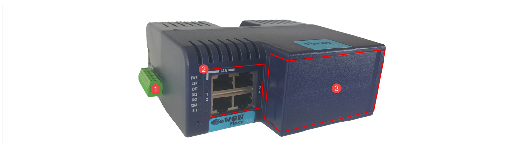
Fig. 2 Modular Concept of the Flexy 205
