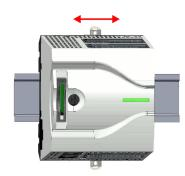
**4.** Move the CPU on the mounting rail at its position.
