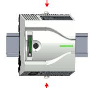
**6.** To fix the CPU at the mounting rail, move the locking levers back to the initial position.
