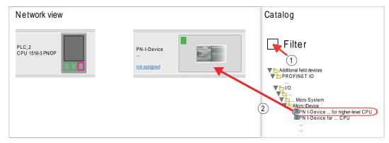
3. To connect to the CPU, click at 'not assigned' and select the PROFINET interface of the CPU.
