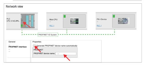
5. Click in the *Network view* at the PN I-Device and switch to the *Device overview*.
