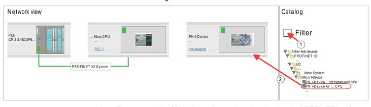
2. To connect to the CPU, click at 'not assigned' and select the PROFINET interface of the CPU.
