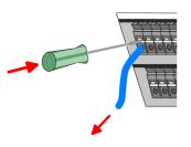
The wire is to be removed by means of a screwdriver with 2.5mm blade width.
