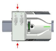
**5.** To fix the extension module at the mounting rail, move the locking levers back to the initial position.
