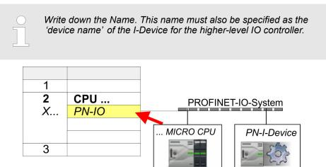
3. For 'PN-IO' at 'slot' 'X...' assign an IP address via the properties dialog.
