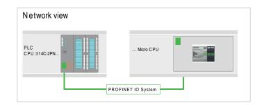
After installing the GSDML the 'PN I-Device for ... CPU' can be found in the hardware catalog at 'Other field devices → PROFINET IO → I/O → VIPA ...
