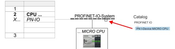
**2.** Open the properties dialog of the PROFINET IO controller of the CPU by a doubleclick at *'PN-IO'* and assign a *'Device name'* for the I-Device in the Register *'General'*.
