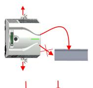
**3.** Pull the locking levers of the CPU outwards until these engage audible.
