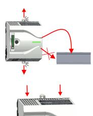
**2.** The CPU has a locking lever on the upper and lower side. Pull these levers outwards as shown in the figure, until these engage audible.
