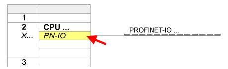
**6.** Use [New] to create a new subnet and assign valid IP address data for your PROFINET system.
