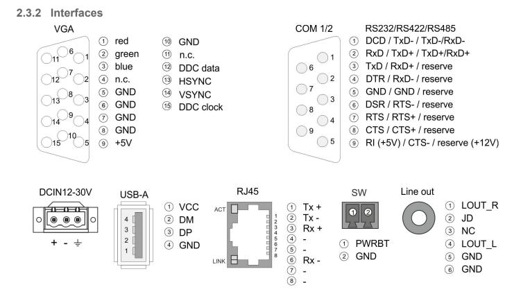
**Power supply** The Panel PC has got an integrated power supply. The power supply has to be provided with DC 12... 30V. For this you find an according DC 24V slot at the back. The power supply is protected against inverse polarity and overcurrent.
