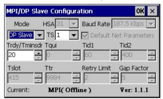
It is possible to set up the DP slave with the tool via software if the hardware of the Touch Panel does not support this. In this case MPI does not work either.
