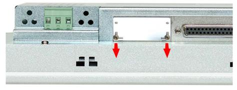
**1.** Remove the cover plate of the COM3 port by removing the screws and pulling the plate.
