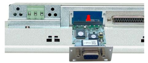
Push the interface module into the opening. Push the interface module in the device until the holding plate fits to the housing. Here the interface module is put into the right position by 2 inner guide rails.
