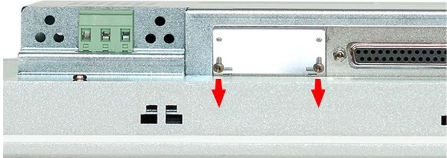
1. Remove the cover plate of the COM3 port by removing the screws and pulling the plate.
