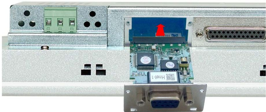
2. For installation insert the interface module into the opening. Push the interface module in the device until the holding plate fits to the housing. Here the interface module is put into the right position by 2 inner guide rails.
