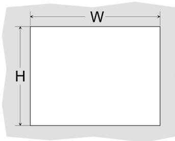
For the installation into a operating tableau and control cabinet fronts, the Touch Panel requires the following front plate cutting:
