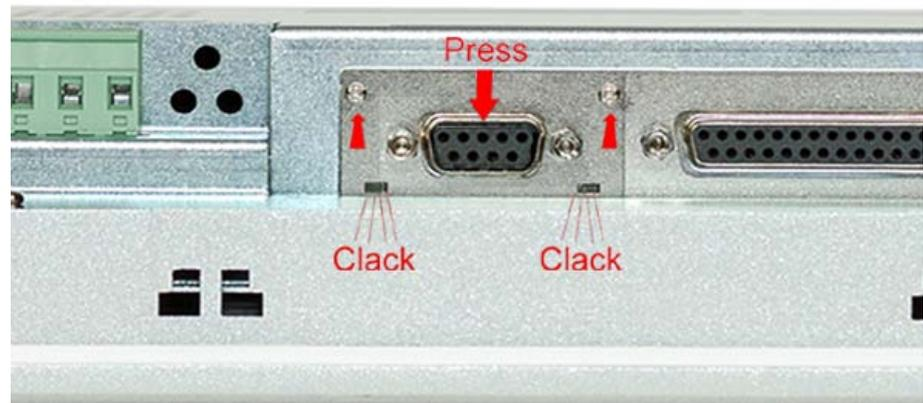
3. ▶ Now press the interface module downwards until the holding plate snaps into the lugs.
