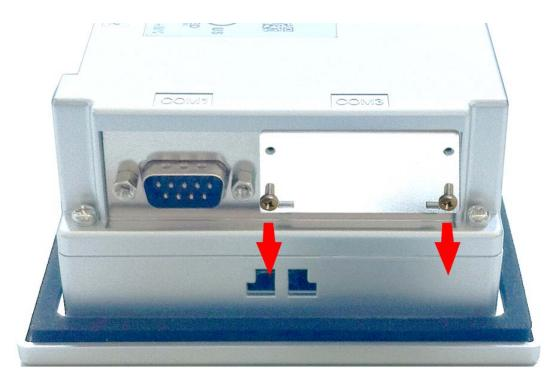
**1.** Remove the cover plate of the COM3 port by removing the screws and pulling the plate.
