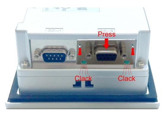
3. Now press the interface module downwards until the holding plate snaps into the lugs.
