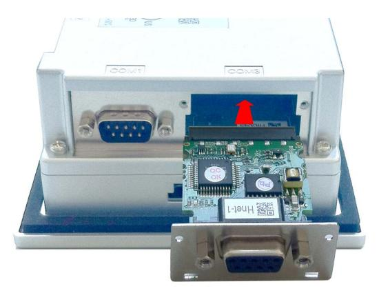
For installation insert the interface module into the opening. Push the interface module in the device until the holding plate fits to the housing. Here the interface module is put into the right position by 2 inner guide rails.
