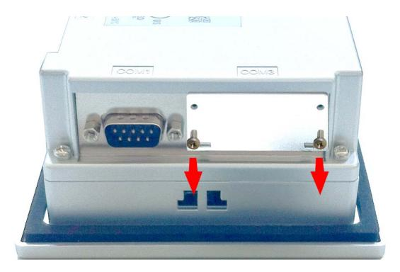
**1.** Remove the cover plate of the COM3 port by removing the screws and pulling the plate.
