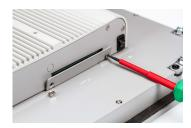
The CFast card slot is located on the rear top side of the Panel PC. It is closed with a cover plate.
