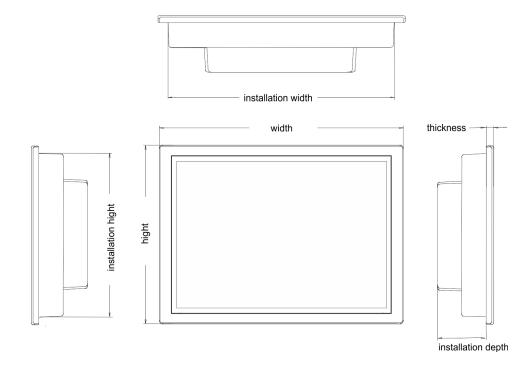
**Installation dimensions** For the installation of the Panel PC in control cabinets and desks the following dimensions are necessary:
