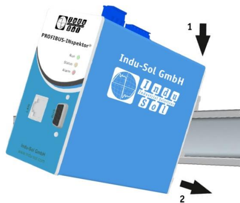
Figure 2: Device installation on top-hat rail
