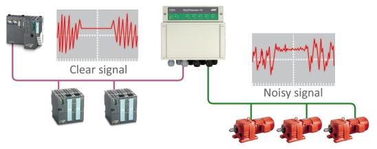
Because of the isolation and intelligence the PROFIBUS-Multi-Repeater provides, it can be used as a barrier for electrically sensitive segments. This keeps the backbone and other Channels clean.
