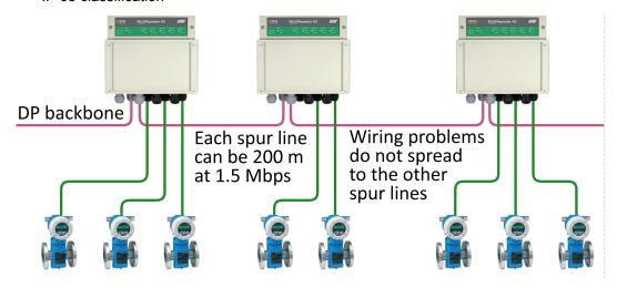
Long spur lines to instruments and the possibility to remove/insert them during operation. Short circuit protection on each spur line is automatically provided.
