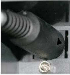
The diagnostics device is directly supplied by the Mini-DIN jack of the IBS master and is ready for operation after connection. Please consider that the arrow on the plug ► shows to the right side when the diagnostics device is connected to the Mini-DIN jack.
