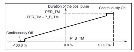
■ Two-Step Control with Monopolar Manipulated Variable Range (0 % to 100 %)
