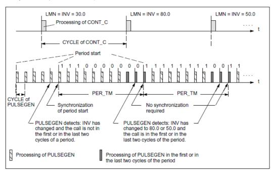
The automatic synchronization can be disabled at the SYN\_ON input (= FALSE).
