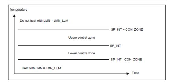
Before activating the control zone manually, make sure that the control zone band is not too narrow. If the control zone band is too small, oscillations will occur in the manipulated variable and process variable.
