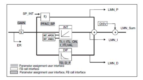
PID Algorithm (*GAIN, TI, TD, D F*)
