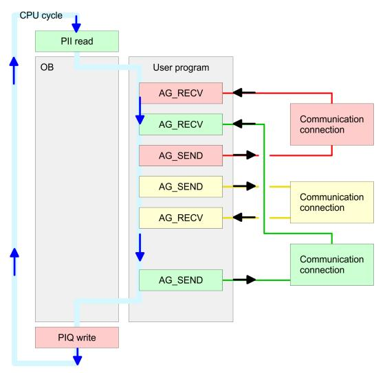
The FC blocks with concerning communication connection are grouped by color. Here you may also see that your user application may consist of any number of blocks. This allows you to send or receive data (with AG\_SEND res. AG\_RECV) event or program driven at any wanted point within the CPU cycle. You may also call the blocks for **one** communication connection several times within one cycle.
