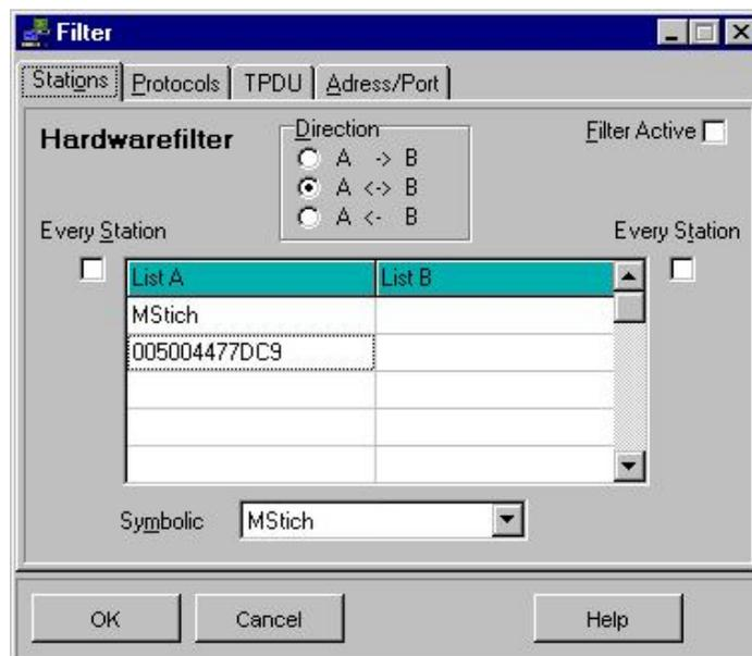
If you wish to enter a station address you must select a list element and enter the respective Ethernet address. If you have activated the symbolism you can select a symbolic name in the selection field which is transferred into the list.
