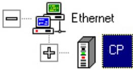
Depending on the firmware of the CP, you may execute a reboot online. As soon as you entered a destination IP address and a valid password, the CP is rebooted with [Apply]. This function is password protected. The password is preset in the register Password.
