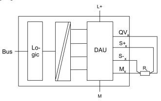
Connecting loads at voltage output at 2-wire cabling
