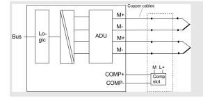
When connecting thermocouples with one compensation slot, you have to regard that the thermocouples have the same type. The compensation slot is to be connected at COMP+ and COMP- and is to be supplied external.
