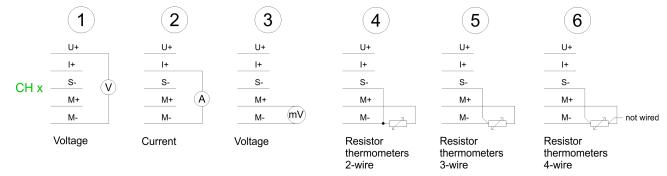
Please take care that the maximum permissible common-mode voltage of 2V between the inputs at connection of voltage and current giver is not exceeded. To avoid wrong measurements you connect the individual connections M- with each other.
