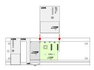
To deploy the SPEED7-CPU exclusively at the SPEED-Bus, plug it between the triangular positioning helps to the slot marked with "CPU SPEED7" and pull it down.
