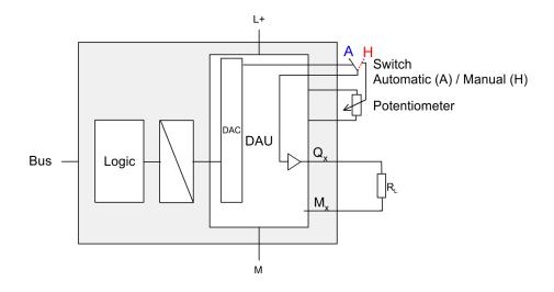
332-5HD50 - AO 4x12Bit I for manual operation > Manual operation
