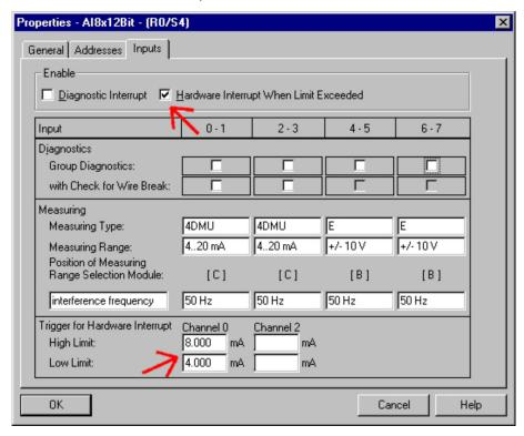
You may activate a process interrupt for channel 0 and 2. Using the default configuration, the process interrupts are not activated.
