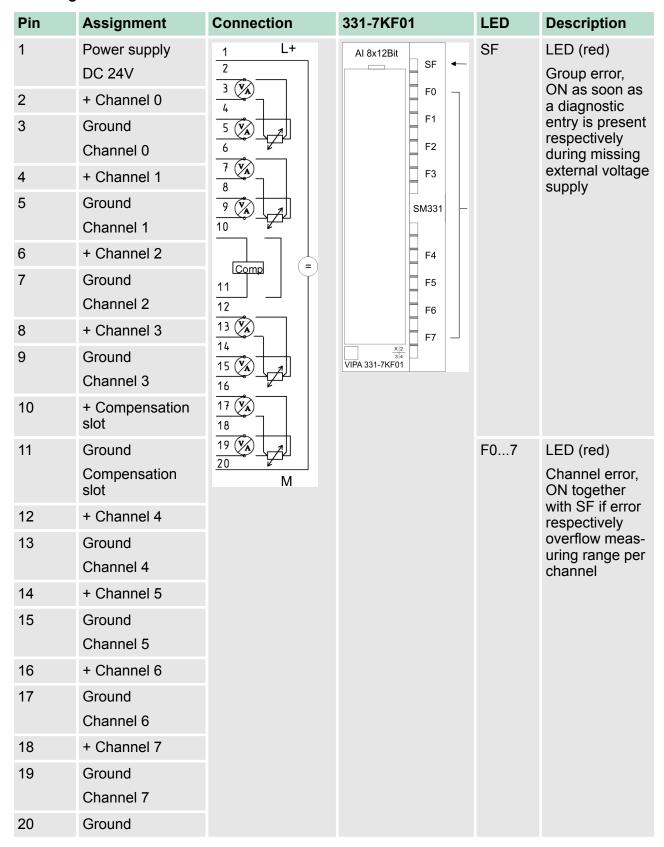
331-7Kx01 - AI 8(2)x12Bit > Connection of sensors
