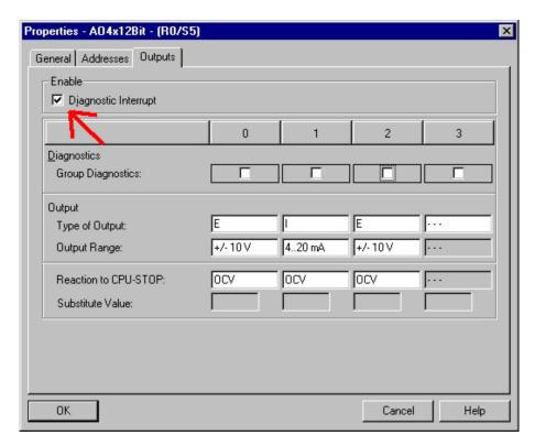
A diagnostic interrupt is only transmitted to the CPU, if you have activated the diagnostic interrupt in the parameterization window. The following errors a diagnosis:
