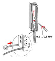
**7.** Fix the cable binder for the cable bundle.
