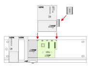
1. If also standard modules shall be plugged, take a bus coupler and click it at the CPU from behind like shown in the picture. Plug the CPU between the triangular positioning helps to the slot marked with "CPU SPEED7" and pull it down.
