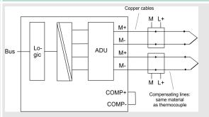
M+: measuring line (positive) COMP+: Compensation connection (positive)
