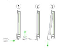
**1.** Dismantle the according protection flaps of the SPEED-Bus slot with a screw driver (open and pull down).
