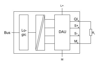
Connecting loads at voltage output at 4-wire cabling (only 332-5Hx01)
