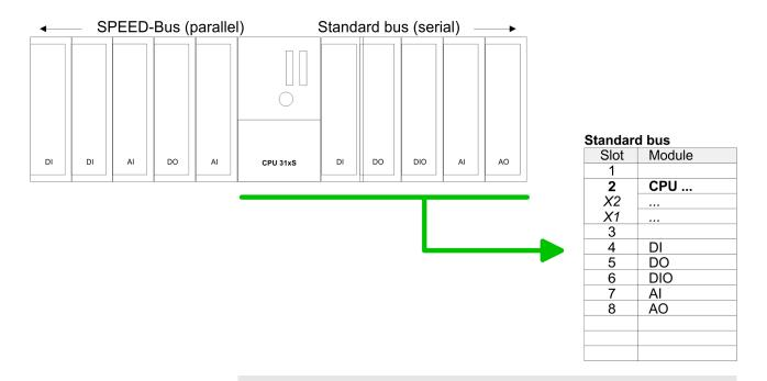
To extend the bus you may use the IM 360 from Siemens where you can connect up to 3 further extension racks via the IM 361. Bus extensions are always placed at slot 3.
