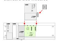
1. If also standard modules shall be plugged, take a bus coupler and click it at the CPU from behind like shown in the picture. Plug the CPU between the triangular positioning helps to the slot marked with "CPU SPEED7" and pull it down.
