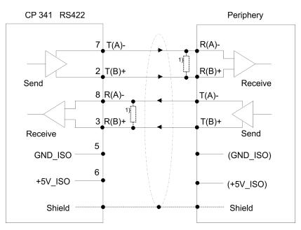
1) In the case of cables > 50m you have to solder in a terminating resistor of approximately  $330\Omega$  on the receiver for data free traffic.
