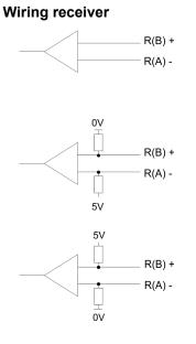
At the CP interface the wiring of the receiver is realized as follows:
