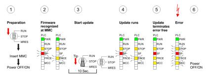
⇒ The update is successful finished when the LEDs PWR, STOP, SF, FRCE and MCC are on.
