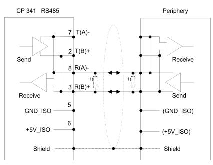
In the case of cables > 50m you have to solder in a terminating resistor of approximately 330Ω on the receiver for data free traffic.
