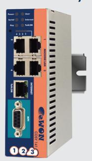
The eWON Cosy (COmmunication made eaSY) is an industrial VPN router that is designed to offer easy remote access, across the Internet, to machines and installations at customers or in the field.
