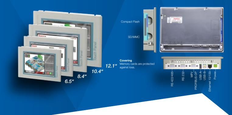
professional Panels – extremely powerful Touch Panels with unique features and high scalability. Offered with or without Movicon 11 runtime and optional RFID module.
