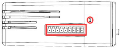
Main connector including power input terminal, 1 DO and 2 DI 1
